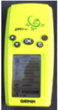
2. Press the down arrow until **units** is highlighted. Press **OK**.
