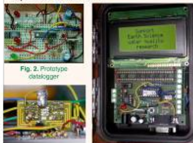
Fig. 3. Bare turbidity, water color and water temperature sensors, before waterproofing with heat shrink tubing and clear epoxy.
