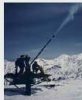
Fig. 6. Use of "avalancher" to release avalanches from distant slopes
