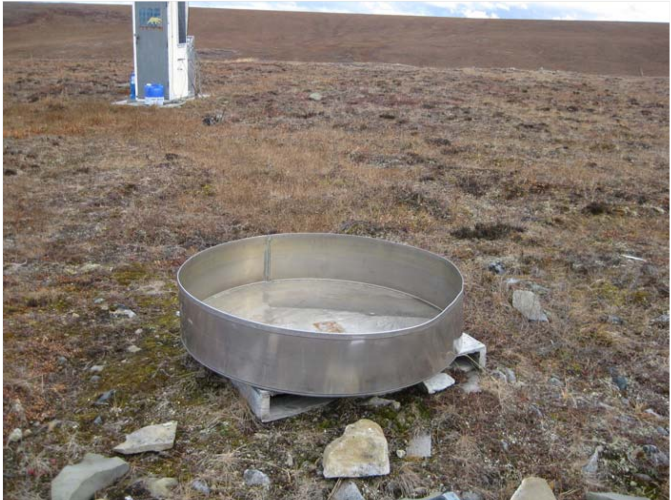
Class A Evaporation Pan located at the Imnavait Creek Basin on the North Slope of Alaska
